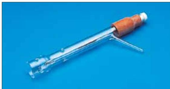
Photograph of a standard hydrogen electrode
