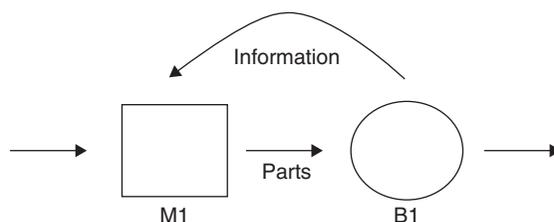
Figure 1.6 Simple kanban system demonstrating feedback
