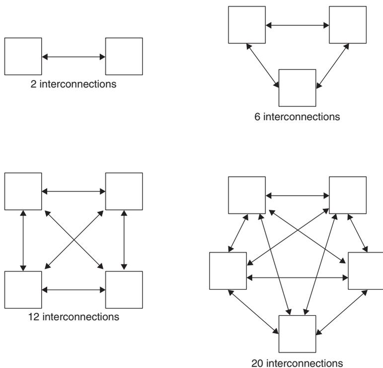
**Figure 1.5** Job shop systems: interconnections and combinatorial complexity
